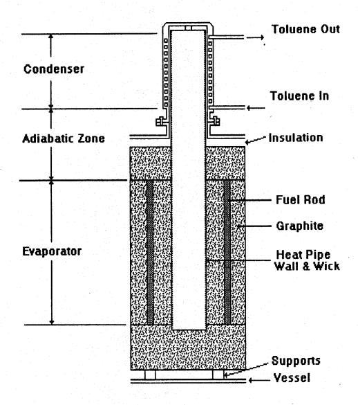
FIGURE 2: A Nuclear Battery Heat Pipe/Vaporizer Assembly
