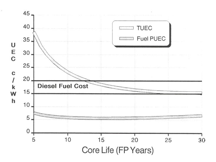
FIGURE 4: Nuclear Battery Lifetime Unit Energy Costs for Electricity
