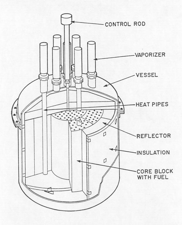
FIGURE 1: Nuclear Battery Reactor Core Module
