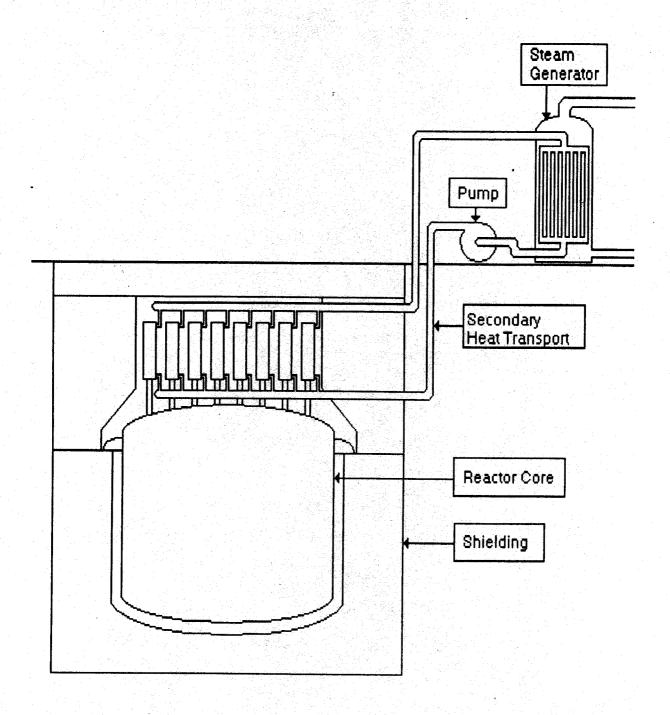
FIGURE 5: Schematic of a 2400-kW(t) Nuclear Battery for Steam Generation
