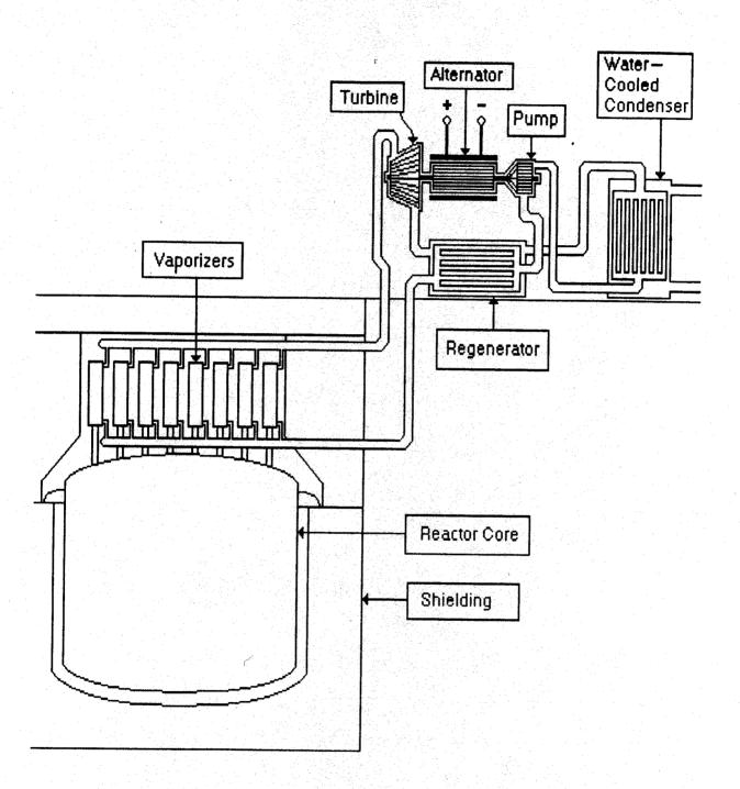
FIGURE 3: Schematic of a 600-kW(e) Nuclear Battery for Village Electricity
